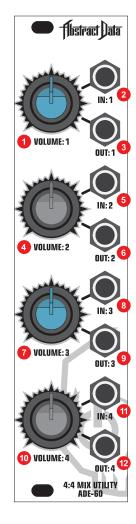
1 VOLUME: 1 Sets the volume and the level of user-defined functions for channel 1
